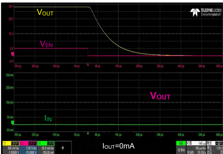
V_{OUT} = 3.3V , V_{IN} = 12V , Power Off
