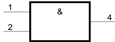
Figure 8-2 IEC logic symbol
