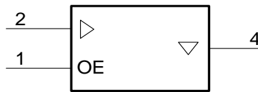
Figure 8-2 IEC logic symbol
