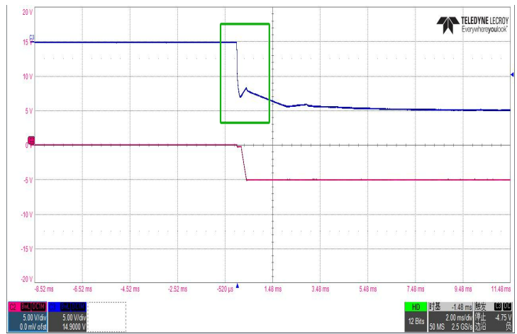
Figure 9-2. Test with the circuit that a 100\mu\text{F} -25V electrolytic capacitor parallel to the C_{IN} [Test Circuit is shown in Figure 9-6]
