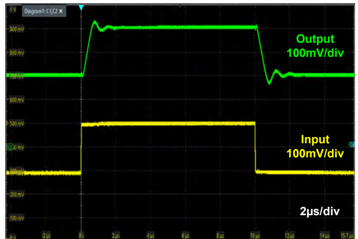
Small-Signal Step Response ( V_S = 15V )
